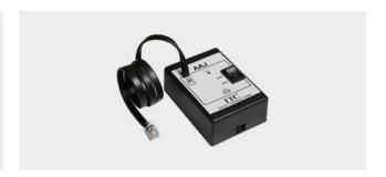
It detects the guest presence in the room by closing of a contact (i.e.: suite control) and activate the related room services. It is installed in the room electric panel and connected to the UGC unit through 6 conductors cable, ending with 6/6 telephone PLUG. Dimensions: 64x89x40mm. Weight 0,1Kg.
